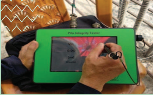
Pile Integrity Test (PIT)
